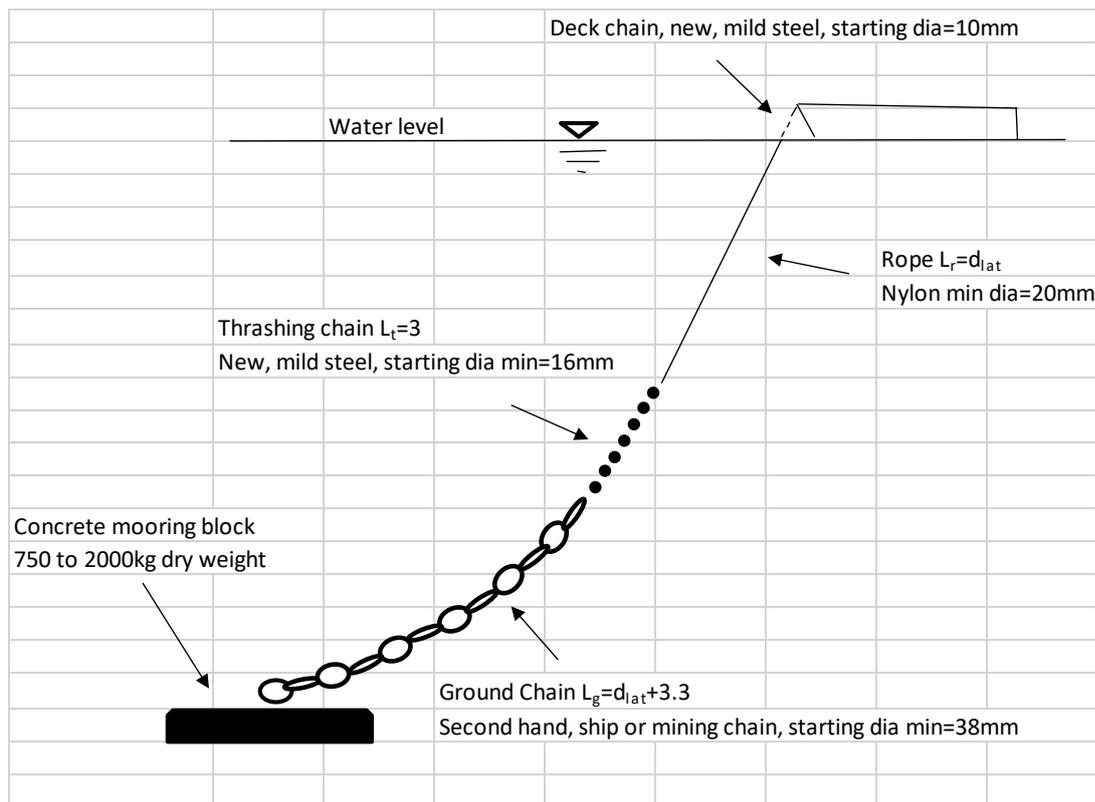
Where:  $L_r$  = length of rope     $L_t$  = length of thrashing chain     $L_g$  = length of ground chain     $d_{lat}$  = depth of water at lowest astronomical tide
